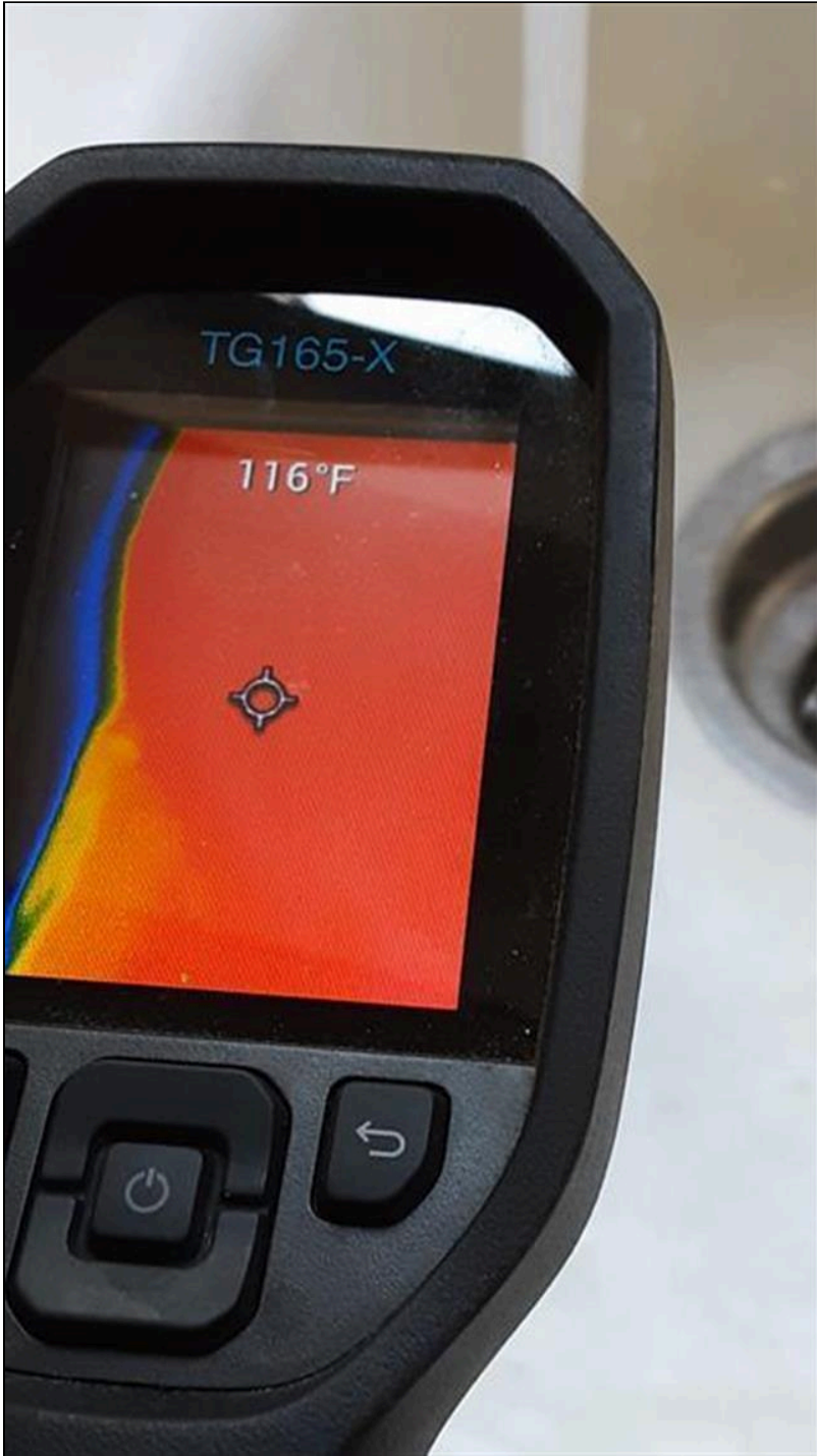
6.2 Item 3(Picture) Hot water temp
