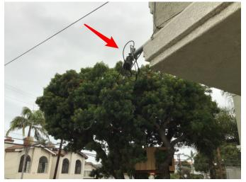
**98:** The overhead service wires are passing through trees or other foliage. We recommend the trees be trimmed clear of the wires or the service be reconfigured. To reduce shock hazard during this procedure, the work should be coordinated with the utility provider.
