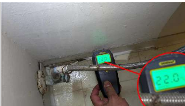
6.4.B Item 7 (Picture) High moisture meter readings noted at lower portion of wall by toilet. (Moisture meter readings were taken as a courtesy and are not part of a general home inspection.
