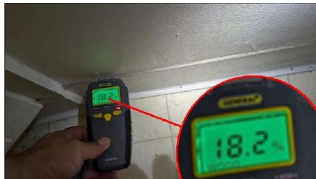
6.4.B Item 8 (Picture) High moisture meter readings noted at lower portion of wall by sink cabinet. (Moisture meter readings were taken as a courtesy and are not part of a general home inspection.
