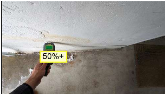
3.2 Item 11 (Picture) High moisture meter readings noted at area of concern. (Moisture meter readings were taken as a courtesy and are not part of a general home inspection.)
