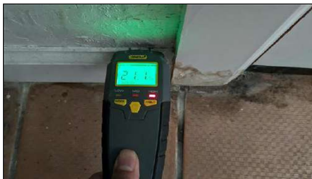
4.0 Item 8 (Picture) Foyer: High moisture meter readings noted at area of concern. (NOTE: Moisture meter readings were taken as a courtesy and are not part of a general home inspection.)
