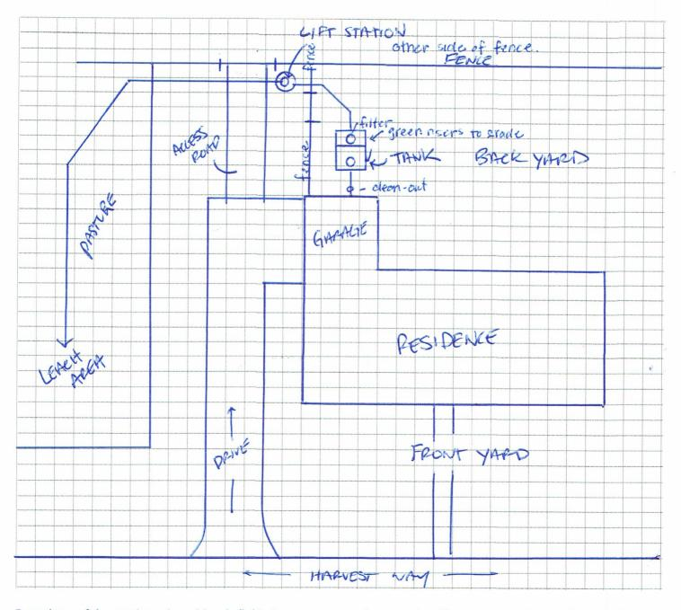
Locations of the septic tank and leach field above are approximate only. The exact location or dimensioning is not within the scope of this inspection. Drawing is not to scale.
