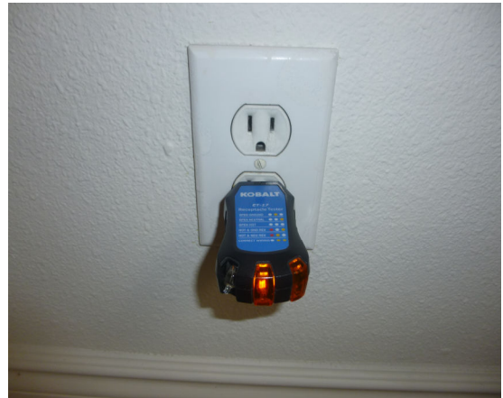
OPEN GROUND ON ALL WALL OUTLETS IN EVERY ROOM THROUGH OUT HOUSE/OUTLET ARE NOT GROUNDED BY TODAY'S STANDARDS RECOMMEND FURTHER EVALUATION
