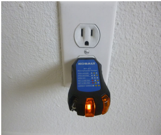
OPEN GROUND ON ALL WALL OUTLETS IN EVERY ROOM THROUGH OUT HOUSE/OUTLET ARE NOT GROUNDED BY TODAY'S STANDARDS RECOMMEND FURTHER EVALUATION
