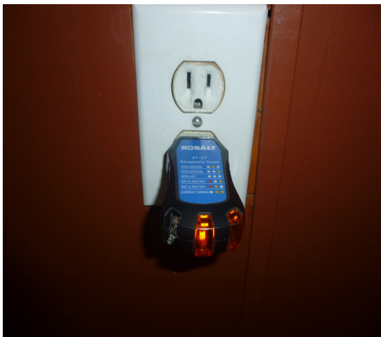
OPEN GROUND ON ALL WALL OUTLETS IN EVERY ROOM THROUGH OUT HOUSE/OUTLET ARE NOT GROUNDED BY TODAY'S STANDARDS RECOMMEND FURTHER EVALUATION
