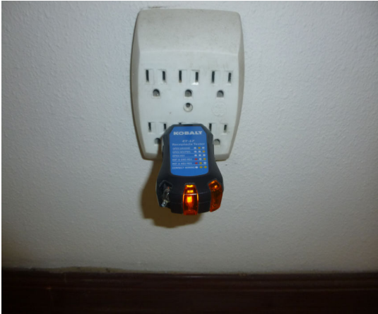
OPEN GROUND ON ALL WALL OUTLETS IN EVERY ROOM THROUGH OUT HOUSE/OUTLET ARE NOT GROUNDED BY TODAY'S STANDARDS RECOMMEND FURTHER EVALUATION
