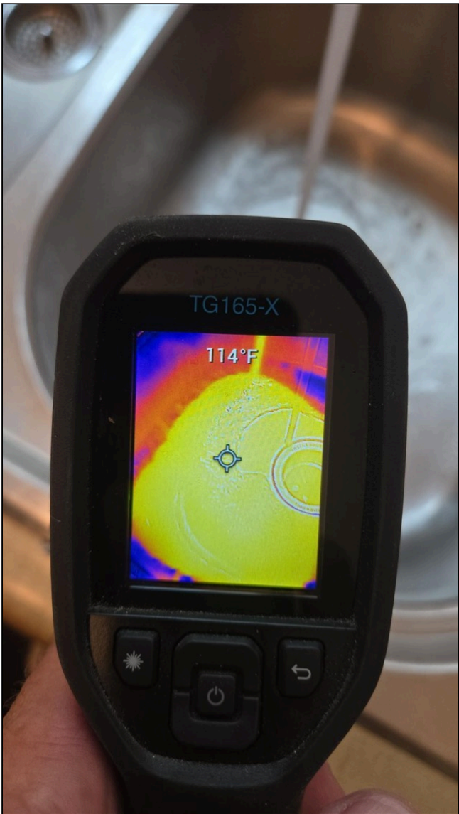
5.2 Item 4 (Picture) Hot water temperature
