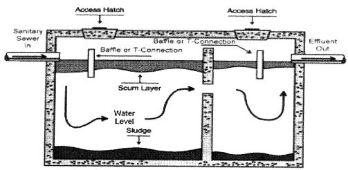
ACCESS HATCH/LID (We check the lids to make sure there are no major cracks and That it fits snug. There needs to be enough lids to access each compartment, and their construction need to be sound and meets code.)
