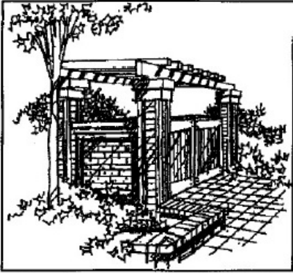
Decorative masonry and metal mixed with wood elements create pleasant trash enclosure
