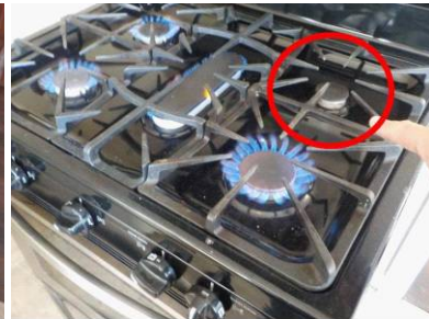
Igniter not functioning - improper
