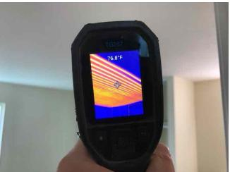
**83:** The ceiling heat system located living room did not respond to normal user controls at the time of inspection and needs to be further evaluated by an appropriate qualified professional.
