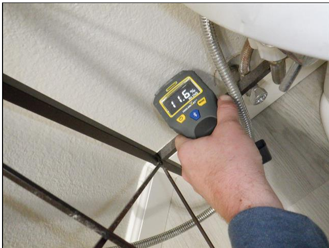
5.1 Item 1(Picture) Moisture test around plumbing fixtures
