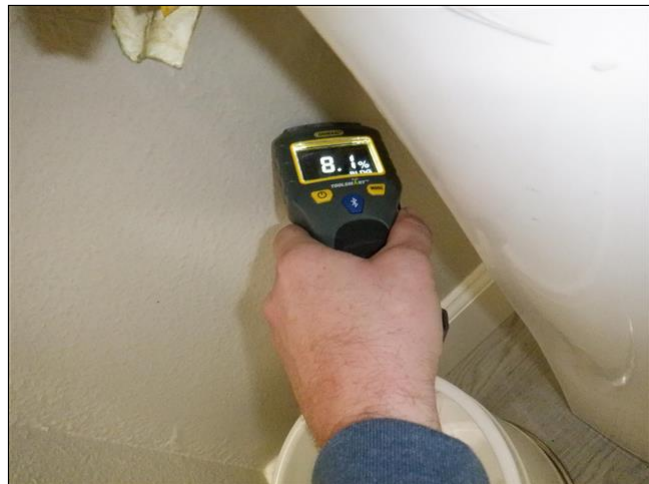
5.1 Item 2(Picture) Moisture test around plumbing fixtures
