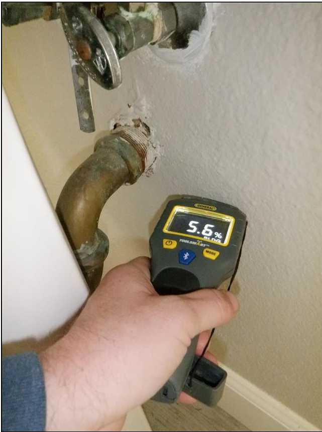
5.1 Item 3(Picture) Moisture test around plumbing fixtures
