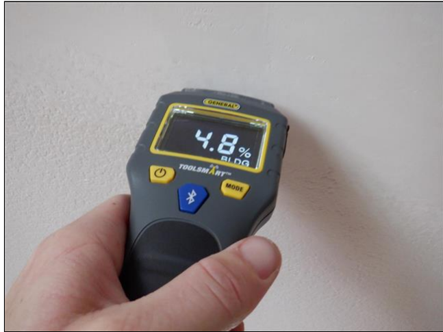
4.0 Item 2(Picture) Moisture test at living room ceiling repair
