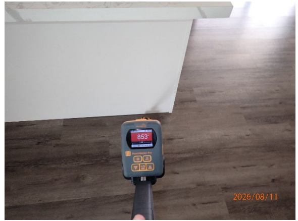
Elevated moisture readings on floor in kitchen
