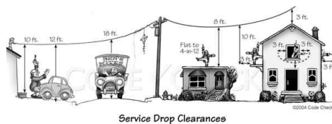
Typical Service Drop Clearance Requirements.
