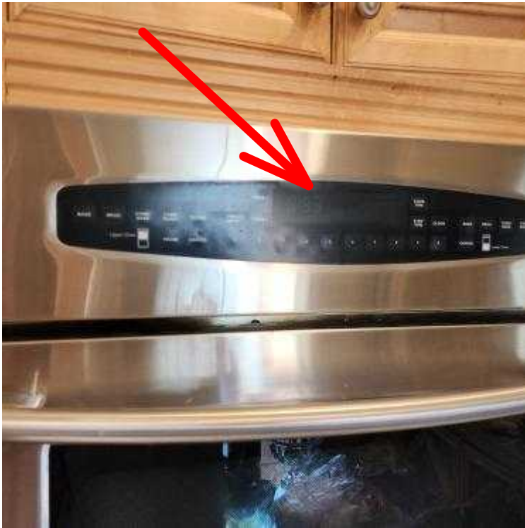
Low visible display on oven control panel
