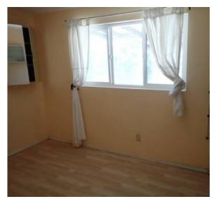
**Safety** - Window(s) did not meet emergency egress requirements at one or more bedrooms. Window sills were slightly higher than the current code requirement, which is a maximum 44" above the floor. Because of the old construction standard (46") and replacement windows, the sill height is now higher than 46" above the floor.
