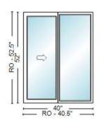
Frame Width = 40, Frame Height = 52, Sash Split = Even Operation / Venting = XO Flush Fin Frame Color = White Double Glaze, SolarTherm Ultra, DS / DS, IE Liners, STC Rating = 31 Lock Height = Standard Lock Height Standard Screen U-Factor = 0.3, CR = 56, SHGC = 0.22, VT = 0.52, CPD = ASO-A-102-09649-00001 Net Overall Line Item Notes:
