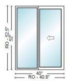
A272-70 Series OX 40 x 52 Frame Width = 40, Frame Height = 52, Sash Split = Even Operation / Venting = OX Flush Fin Frame Color = White Double Glaze, SolarTherm Ultra, DS / DS, IE Liners, STC Rating = 31 Lock Height = Standard Lock Height Standard Screen U-Factor = 0.3, CR = 56, SHGC = 0.22, VT = 0.52, CPD = ASO-A-102-09649-00001 Net Overall Line Item Notes:
