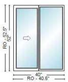
Frame Width = 40, Frame Height = 52, Sash Split = Even Operation / Venting = XO
