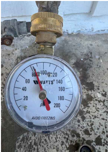
Water Pressure Gauge used
