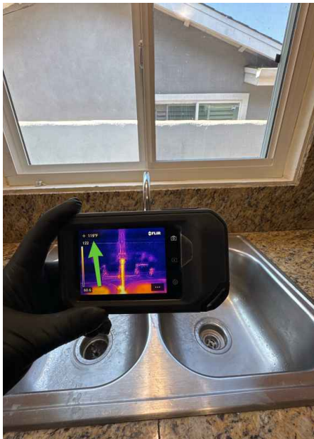
Thermal Image of hot water
