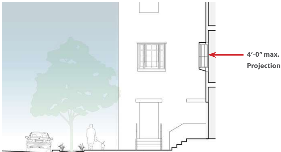
Figure 6.3.5 Bay Window Section
